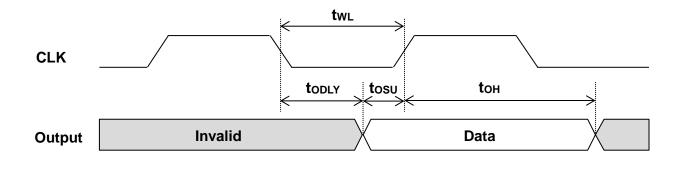
Figure 2 Output timing
