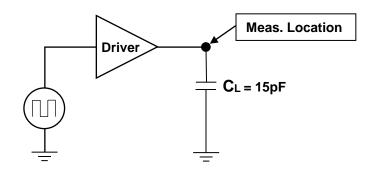
Note 1: C<sub>L</sub> is total equivalent lumped capacitance for each Driver.
