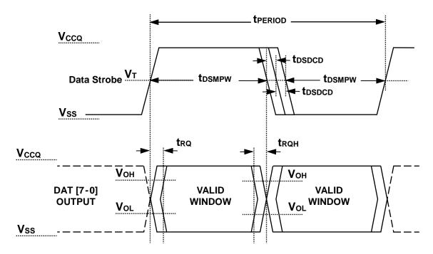
Note:  $V_T = 50\%$  of  $V_{CCQ}$  indicates clock reference point for timing measurements.
