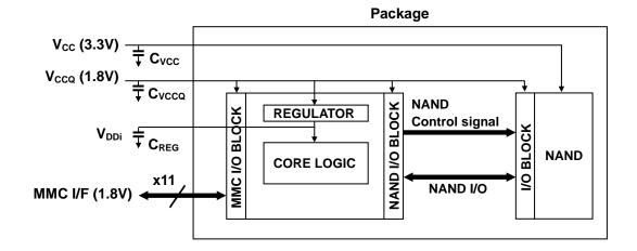
Figure 1 THGAMRG9T23BAIL Block Diagram
