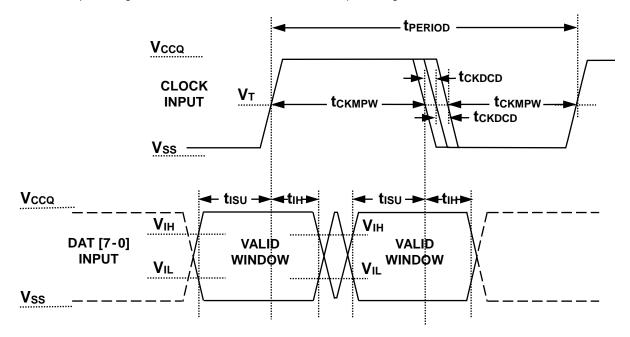
Note:  $V_T = 50\%$  of  $V_{CCQ}$  indicates clock reference point for timing measurements.
