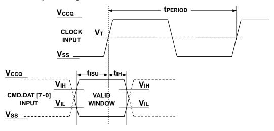
Note 1:  $t_{\text{ISU}}$  and  $t_{\text{IH}}$  are measured at  $V_{\text{IL}}(\text{max.})$  and  $V_{\text{IH}}(\text{min.})$ .
